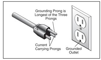
Figure 2. Typical 5-15 plug and receptacle.
